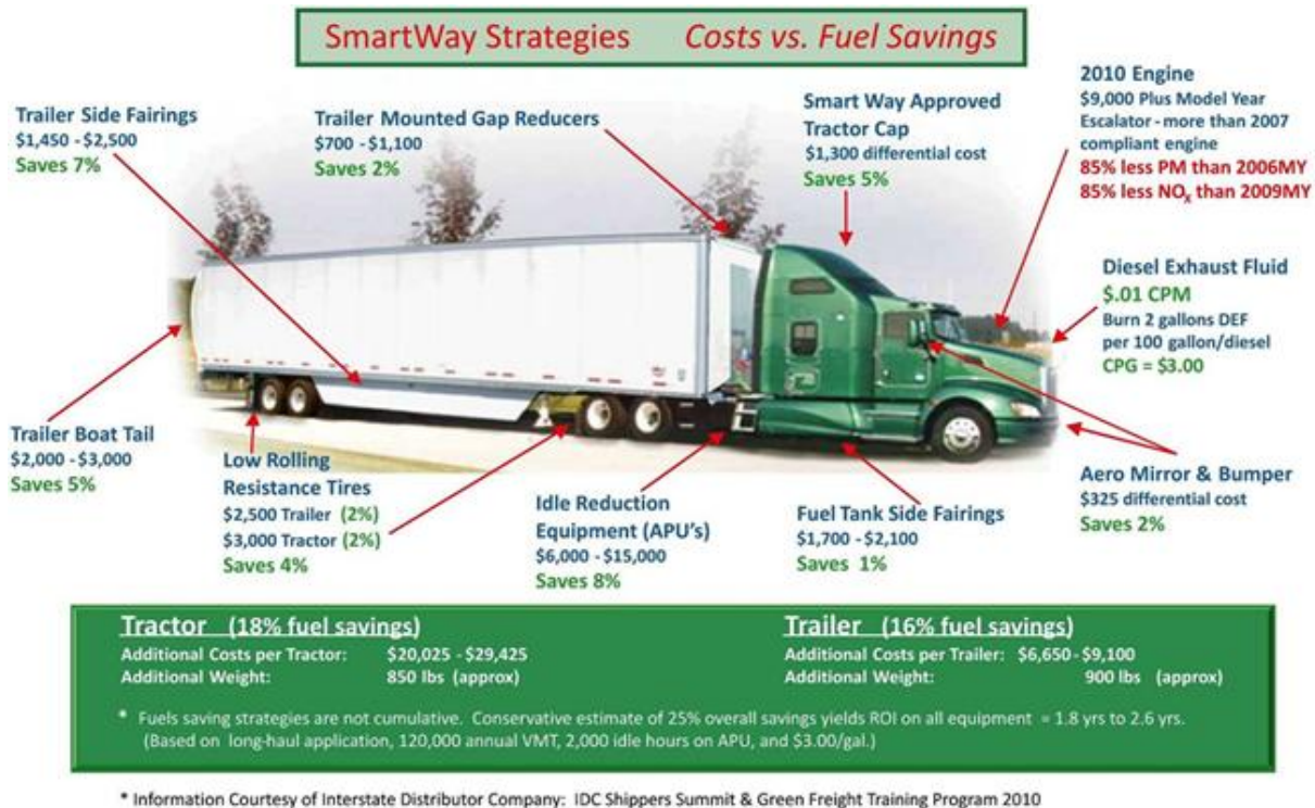
Figure 8. Strategies for saving costs while improving fleet truck fuel efficiency and reducing PM emissions (based on the experience of EPA’s SmartWay Program). Source: [39].
